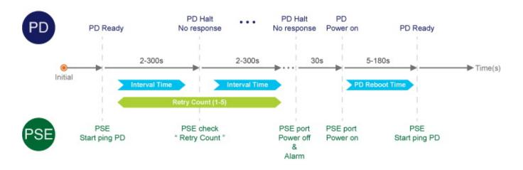
This page provides you how to configure PD Alive Check. The screen in Figure 4-7-8 appears.
