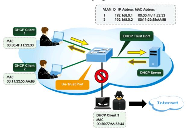
Configure DHCP Snooping on this page. The DHCP Snooping Configuration screen in Figure 4-6-6 appears.
