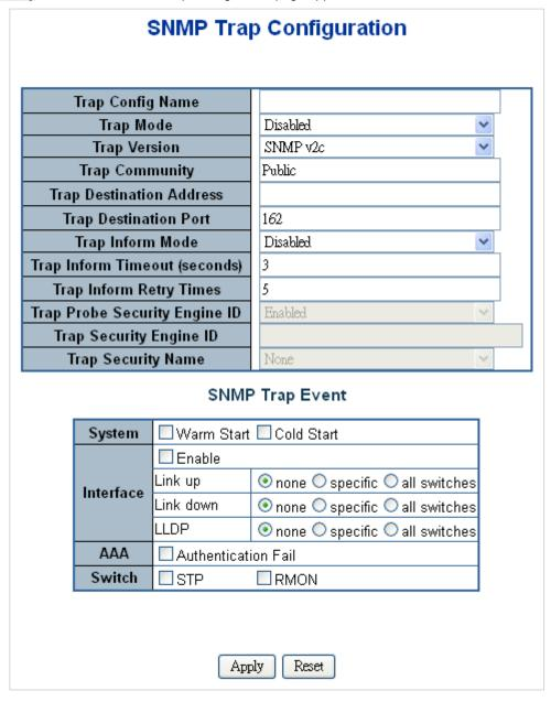
Figure 4-2-2-4-2: SNMP Trap Configuration Page Screenshot
