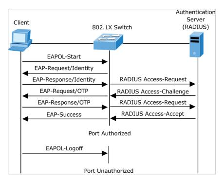
Figure 4-5-2: EAP Message Exchange
