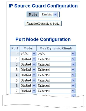
Figure 4-6-7-1: IP Source Guard Configuration Screen Page Screenshot
