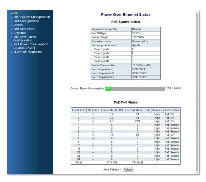
Figure 4-7-1: Power over Ethernet Status
