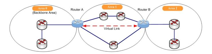
Following is OSPF virtual link configuration table. The virtual link is established between 2 ABRs to overcome that all the areas have to be connected directly to the backbone area. The screen in Figure 4-4-5-8 appears.
