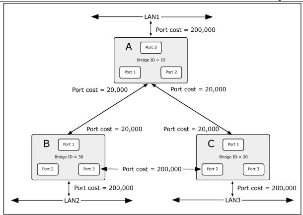
Figure 4-3-10-1-2: Before Applying the STA Rules
