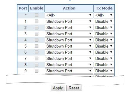
Figure 4-3-16-1: Loop Protection Configuration Page Screenshot
