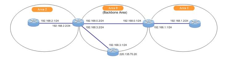
Following is OSPF area configuration table. It is used to specify the OSPF enabled interface(s). When OSPF is enabled on the specific interface(s), the router can provide the network information to the other OSPF routers via those interfaces. The screen in Figure 4-4-5-2 appears.
