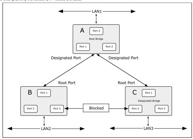
Figure 4-3-10-1-3: After Applying the STA Rules
