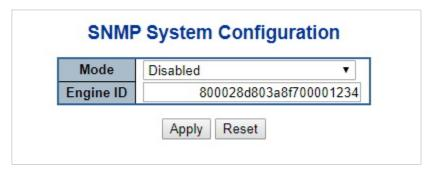
Figure 4-2-2: SNMP System Configuration Page Screenshot
