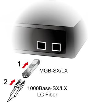
Figure 2-2-4: Plugging in the SFP/SFP+ Transceiver
