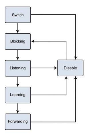
Figure 4-3-10-1-1: STP Port State Transitions
