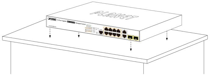
Figure 2-2-1: Place the Managed Switch on the Desktop
