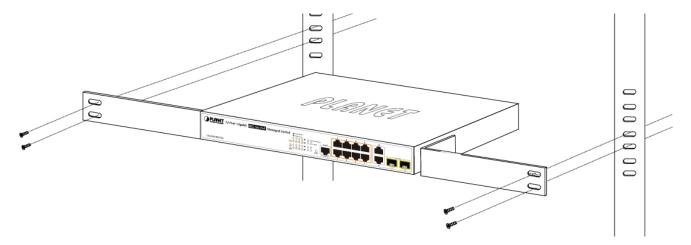
Figure 2-2-3: Mounting Managed Switch in a Rack
