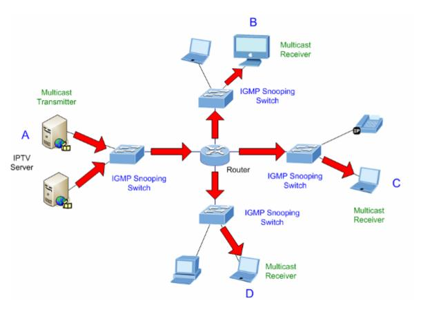
IGMP Snooping Multicast Stream Control
