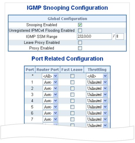
Figure 4-3-11-3: IGMP Snooping Configuration Page Screenshot
