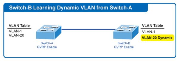
VLANs are **dynamically** configured based on **join messages** issued by host devices and propagated throughout the network.
