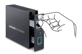
**Step 2:** Remove a blank faceplate from an empty expansion slot on the front of the chassis. The Smart Media Converter board can be installed in any expansion slot.
