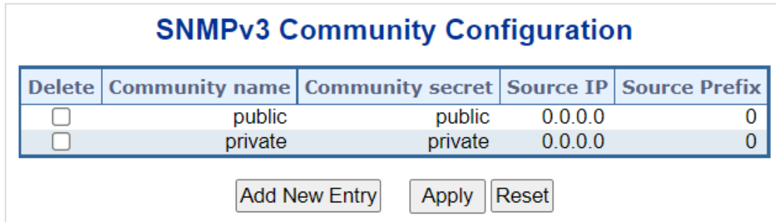
Figure 4-2-2-5: SNMPv3 Communities Configuration Page Screenshot
