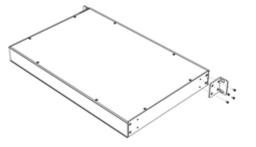
Step 3 Place the device in the rack; adopt 4 bolts to fix two sides mounting lugs in the rack.
