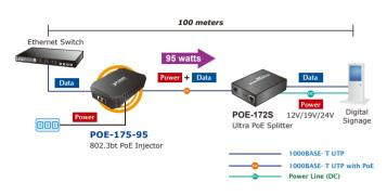
Figure 3: Architecture of connected POE-175-95 and POE-172S
