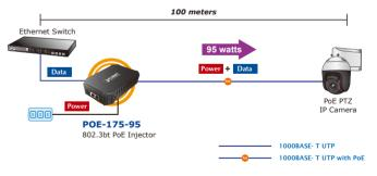
Figure 2: Architecture of connected IEEE 802.3at/bt device
