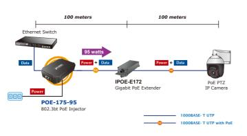
Figure 4: Architecture of connected POE-175-95 and IPOE-E172
