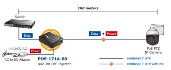
Figure 3: Architecture of Connected IEEE 802.3af/at/bt Devices
