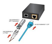
Figure 5-1: GTP-805A Installation
