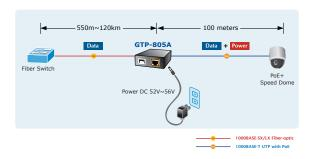
For the places hard to find the power inlet, the GTP-805A provides the easiest way to power your Ethernet devices such as PLANET IEEE 802.3at/802.3af Power over Ethernet Splitter (POE-161S/162S) with Internet Camera or PoE Wireless Access Point installed in a wide-ranging place.
