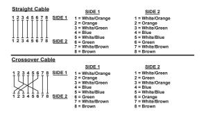
Figure A-1: Straight-through and Crossover Cables
