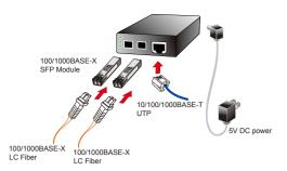
Figure 5: GT-1205A Gigabit Media Converter Standalone Installation
