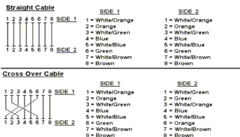
Figure A-1: Straight-Through and Crossover Cable
