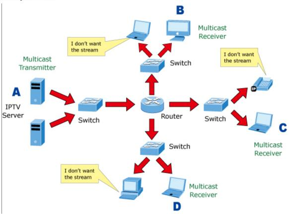
Figure 4-8-2: Multicast Flooding
