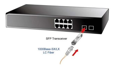
Figure 2-24 Plug-in the SFP transceiver
