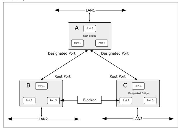
Figure 4-7-3: After Applying the STA Rules
