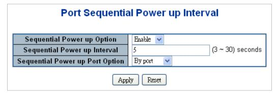
Figure 4-16-3: PoE Port Sequential Power Up Interval Configuration Screenshot
