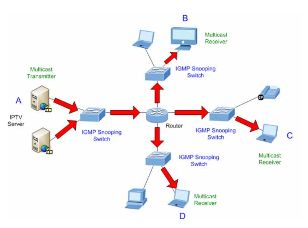
Figure 4-8-3: IGMP Snooping Multicast Stream Control
