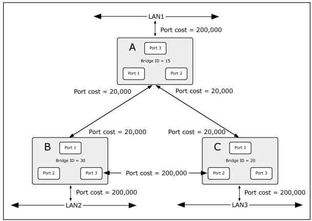
Figure 4-7-2: Before Applying the STA Rules
