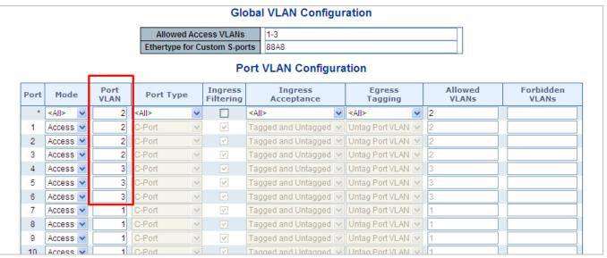
Figure 4-6-9: Change Port VLAN of Port 1~3 as VLAN2 and Port VLAN of Port 4~6 as VLAN3
