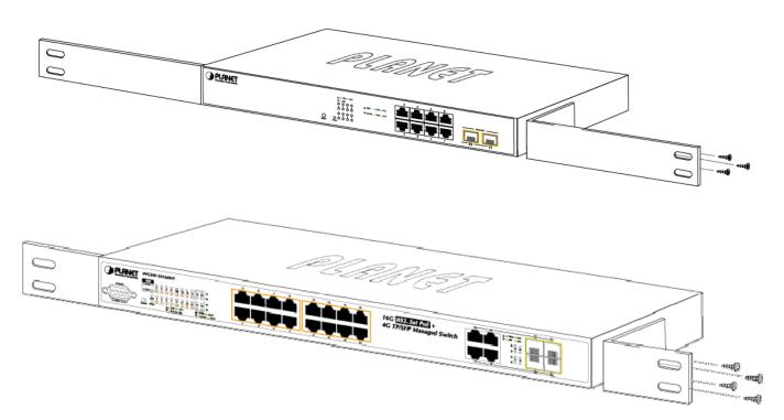
Figure 2-22 Attach brackets to the Managed Switch.
