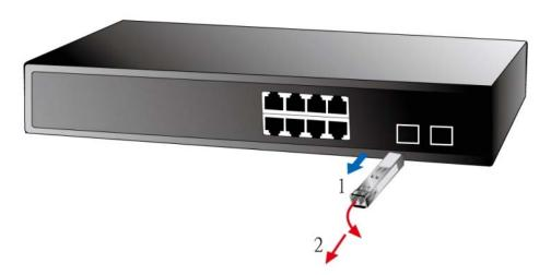
Figure 2-25 Pull out the SFP transceiver
