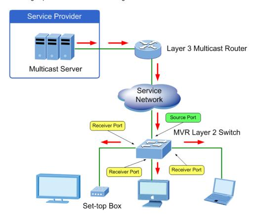
This page provides MVR related configuration. The MVR screen in Figure 4-8-19 appears.
