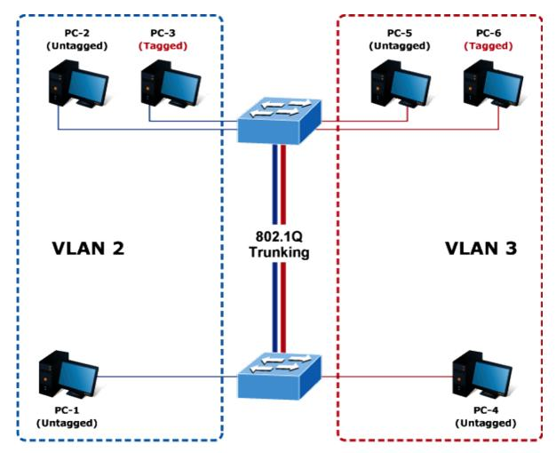
Figure 4-6-11: VLAN Trunking Diagram
