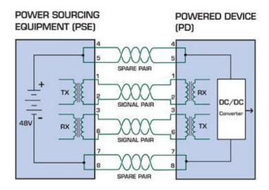
Figure 5-1-1 - Power Supplied over the Spare Pins
