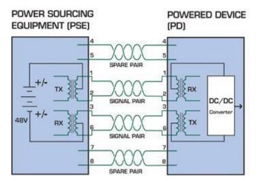
Figure 5-1-2 - Power Supplied over the Data Pins
