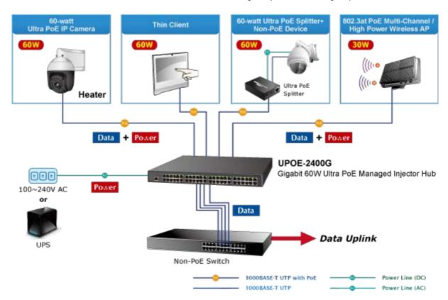
Figure 2-2-4: Network application installation
