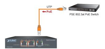
Step 2: The PSE delivers both Ethernet Data and PoE power over UTP cable to the Gigabit PoE Extender and the "PoE-in-use" and "LNK/ACT LED" will be lit steadily.
