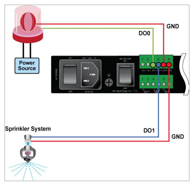
Figure 2-8 Wires DO0 and DO1 to Open Detector
