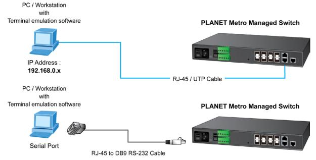
Figure 3-1: Remote Telnet and Console Port Interface Management
