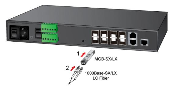
Figure 2-9: Plugging in the SFP Transceiver
