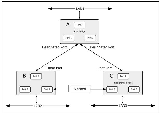
Figure 4-7-3: After Applying the STA Rules
