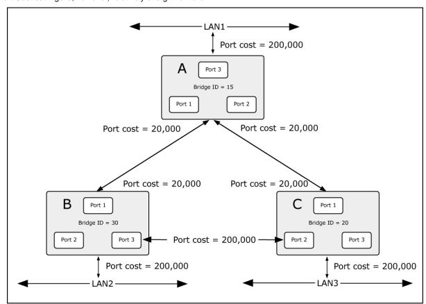
Figure 4-7-2: Before Applying the STA Rules
