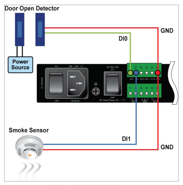
Figure 2-7 Wires DI0 and DI1 to Open Detector
