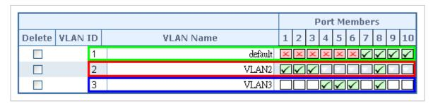
Figure 4-6-12: VLAN overlap port setting & VLAN 1 - The Public Area Member Assign
