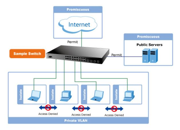
For private VLANs to be applied, the switch must first be configured for standard VLAN operation. When this is in place, one or more of the configured VLANs can be configured as private VLANs. Ports in a private VLAN fall into one of these two groups:
