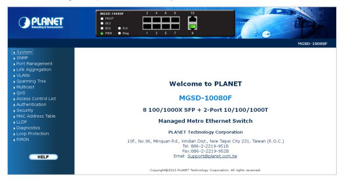
Figure 3-4: Web Main Screen of Managed Switch
