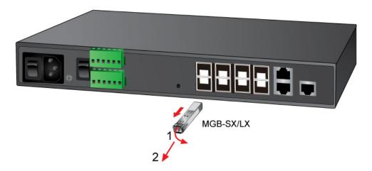
Figure 2-10: How to Pull Out the SFP Transceiver Module
