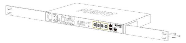
Figure 2-5 Attach Brackets to the Managed Switch.
