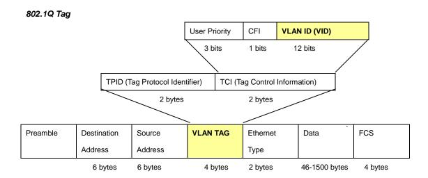
The Ether Type and VLAN ID are inserted after the MAC source address, but before the original Ether Type/Length or Logical Link Control. Because the packet is now a bit longer than it was originally, the Cyclic Redundancy Check (CRC) must be recalculated.
