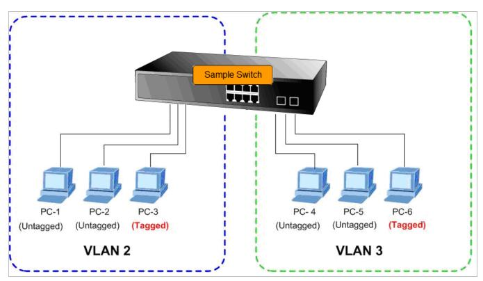
Figure 4-6-8: Two Separate VLAN Diagrams
