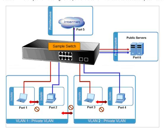
Figure 4-6-14: The Port Isolate VLAN Diagram
