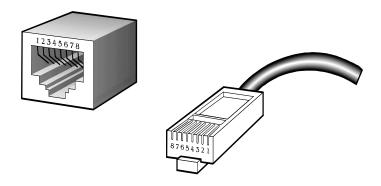
The standard RJ-45 receptacle/connector
