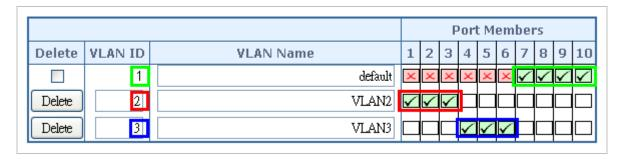
Figure 4-6-9: Add new VLAN group, assign VLAN members for VLAN 2 and VLAN 3 and remove specified ports from VLAN 1 member
