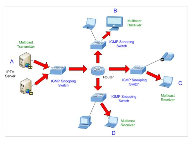
Figure 4-8-3: IGMP Snooping Multicast Stream Control
