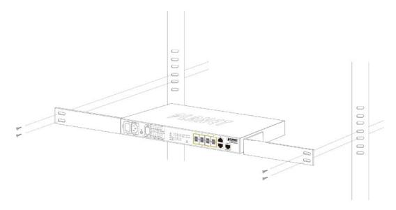
Figure 2-6 Mounting the Managed Switch on a Rack
