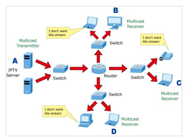
Figure 4-8-2: Multicast Flooding
