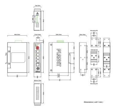
Figure 2-1: IVC-234GT Three-View Diagram
