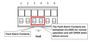
Insert the wires into the fault alarm contacts
