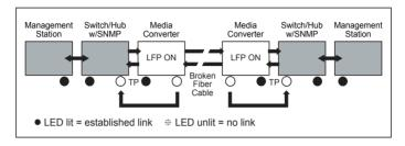
The converter is shipped with the default LFP (LLCF/ LLR) function disabled. This feature can also be turned on on-purpose. If you are familiar with the network installation and for diagnostic purpose (i.e. check which end is broken), you can turn it on and the converter will take effect immediately. Otherwise, please put it in the default position.
