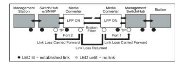
The converter is shipped with the default LFP (LLCF/ LLR) function which is disabled. This feature can also be turned on on-purpose. If you are familiar with the network installation and for diagnostic purpose (i.e. check which end is broken), you can turn it on and the converter will take effect immediately. Otherwise, please put it in the default position.
