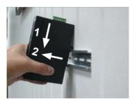
**Step 5:** Lightly pull out the lower part of the DIN-rail bracket to remove it from the track.
