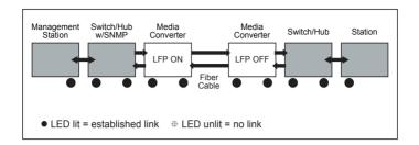
If one of the optical conductors is bad (as shown in the diagram box below), the converter with LLR enabled will return a no-link condition to its link partner. With LLCF also default enabled, the no-link condition is carried forward to the switch/hub where a trap is generated to the management station, and the administrator can then determine the source of the loss.
