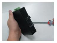
Step 1: Screw the DIN-rail bracket on the Industrial 802.3at PoE Media Converter.
