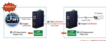
LFP function is turned off by default. This feature can also be turned on via the DIP switch. If you are not familiar with the network installation and for diagnostic purpose (i.e. check which end is broken), you can turn it on. Otherwise, please remain it in the default position.
