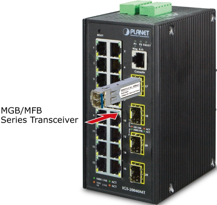
Figure 2-11: Plug in the SFP/SFP+ Transceiver
