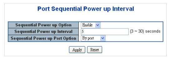
Figure 4-6-1-5: PoE Port Sequential Power Up Interval Configuration Screenshot
