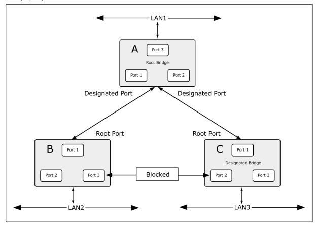
Figure 4-3-4-3: After Applying the STA Rules
