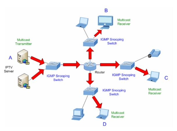
Figure 4-3-5-3: IGMP Snooping Multicast Stream Control
