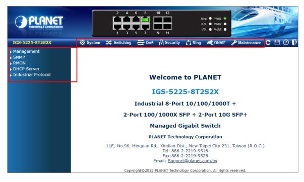
Figure 4-1-5: Industrial Managed Switch Main Functions Menu
