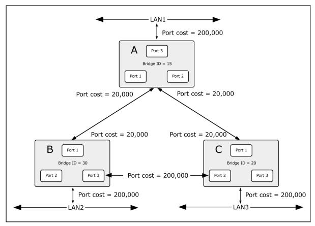
Figure 4-3-4-2: Before Applying the STA Rules
