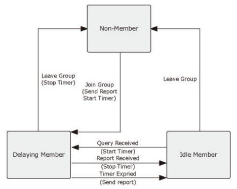
Figure 4-3-5-4: IGMP State Transitions
