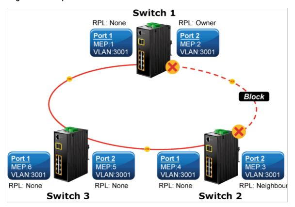
Figure 4-7-1-6: Ring Example Diagram
