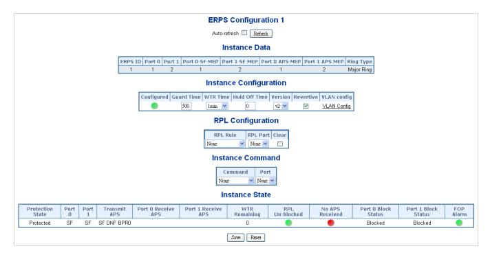
Figure 4-7-1-4: Ethernet Ring Protocol Switch Configuration page screenshot
