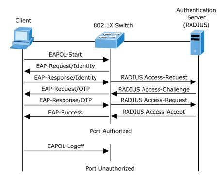
Figure 4-5-2-2: EAP Message Exchange
