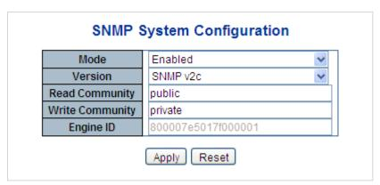
Figure 4-2-2: SNMP System Configuration Page Screenshot
