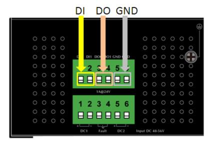
Figure 2-7 Wiring the Redundant Power Inputs
