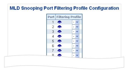
Figure 4-3-6-3: MLD Snooping Port Group Filtering Configuration Page Screenshot
