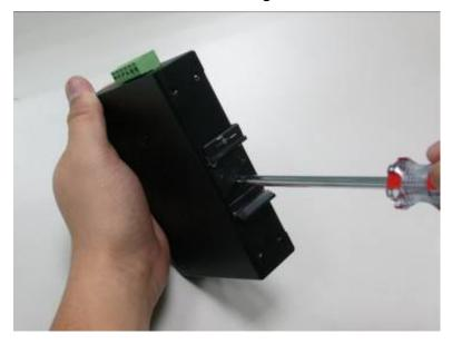
Step 2: Lightly place the upper bracket into the DIN rail and push the unit down till the lower bracket is locked into the track.
