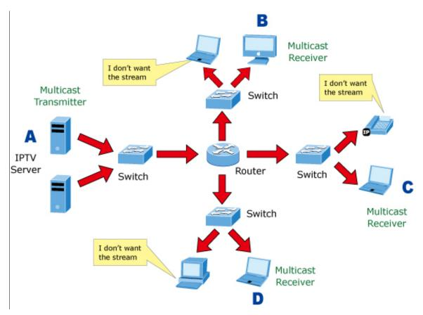
Figure 4-3-5-2: Multicast Flooding
