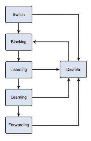
Figure 4-3-4-1: STP Port State Transitions
