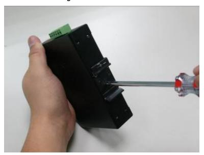
Step 2: Lightly slide the DIN rail into the track.
