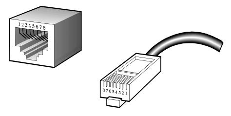
The standard RJ45 receptacle/connector
