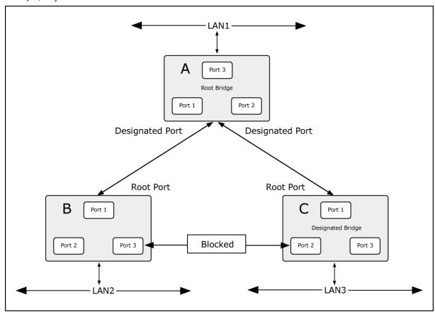
Figure 4-6-3: After Applying the STA Rules
