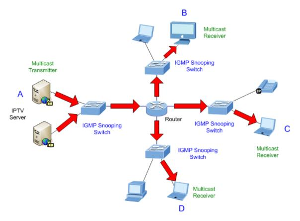
Figure 4-7-5: IGMP Snooping Multicast Stream Control
