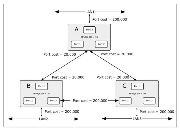
Figure 4-6-2: Before Applying the STA Rules
