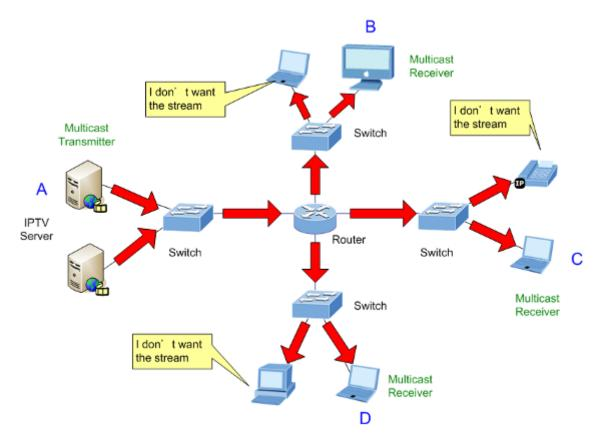
Figure 4-7-4: Multicast Flooding
