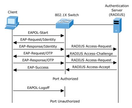
Figure 4-9-2: EAP Message Exchange
