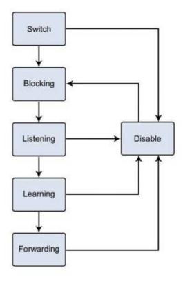
Figure 4-6-1: STP Port State Transitions
