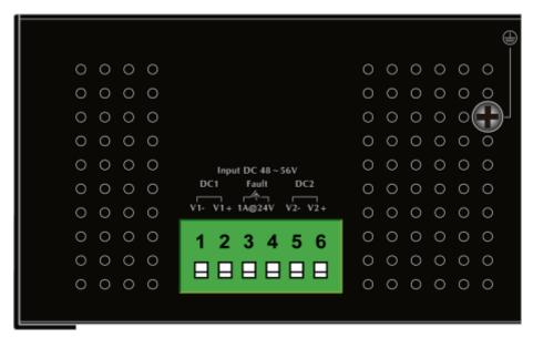
Figure 2-1-4a: Industrial Managed Switch Upper Panel.
