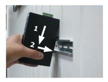
Step 3: Make sure if the DIN-rail is tightly secured on the track.
