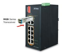
Figure 2-3: Plug-in the SFP Transceiver
