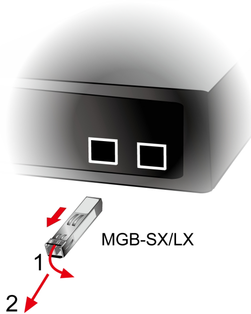
Figure 2-5: How to Pull Out the SFP/SFP+Transceiver
